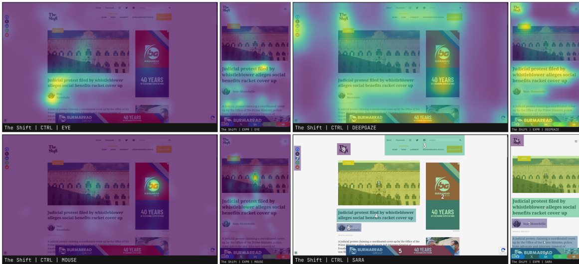
Fig. 6. The Shift interface heatmaps. Within each pair, the control group is on the left and the experimental group is on the right. Top-left: heatmaps from the eye-tracking experiment; bottom-left: heatmaps from the mouse-tracking experiment; top-right: saliency maps generated by DeepGaze IIE; bottom-right: the corresponding SaRa ranks.
